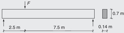
A simply supported glulam beam (GL32c) with cross-section dimensions  $115 \times 700$  mm has a length of 10 m. The load is a short-term load  $F$  acting on the top of the beam. The ends of the beam are restrained against torsion.
