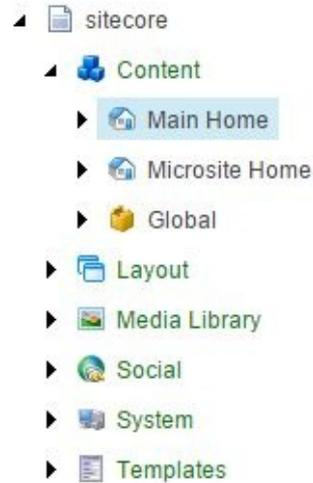
*Figure 7-4. An example of a global tree from Sitecore — this system stores almost every bit of data in a tree structure, including templates and system settings*
