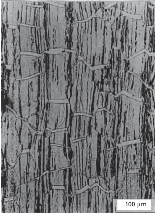
2.6 The appearance of a Mg–0.55% Zr alloy after creep testing at a low stress under conditions corresponding to diffusion creep, showing the development of denuded zones along the transverse grain boundaries and boundary offsets in the longitudinal hydride stringers (the tensile axis is vertical). 29 (courtesy of Langdon).
