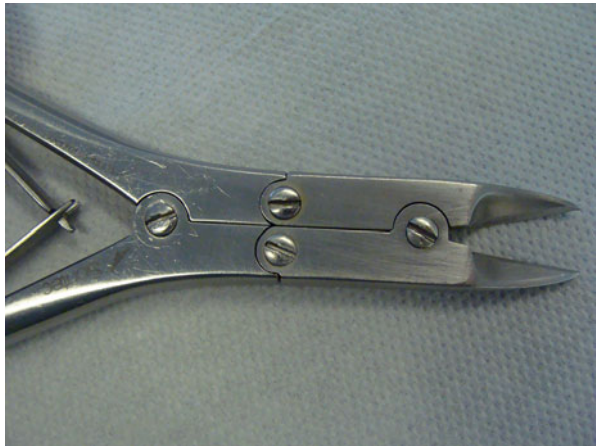
Fig. 1.12 Dual action nail nippers. Note the four hinges making these nippers very powerful
