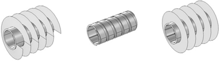
Fig. 3.88 Inner and outer fins and grooves of a cylindrical pipe schematic
