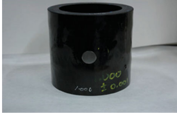
Fig. 3.83 Fiber composite compression cylinder with 1.0-in. diameter pin
