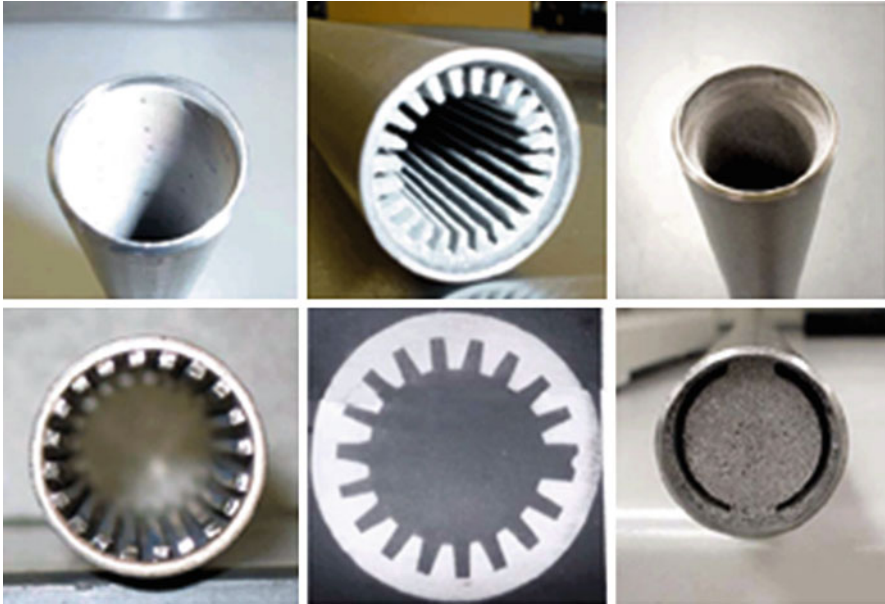
Fig. 2.36 Survey of wick structures produced in titanium and Monel which shows equivalence to structures currently produced in copper
