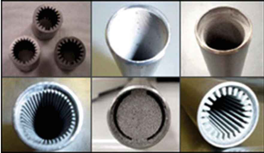
Fig. 2.35 Various wicks for high-temperature water heat pipes
