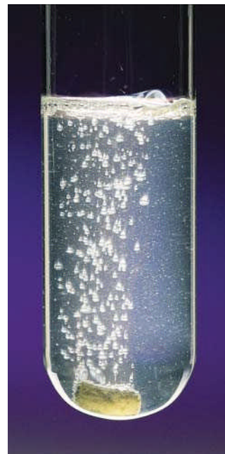
Methanol reacts with sodium metal to give sodium methoxide along with the evolution of hydrogen gas.
