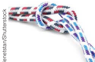
The fibers of this rope are made from nylon 66, a material synthesized from adipic acid.
