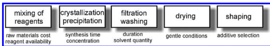
Scheme 1. A simplified overview of processing steps important in industrial MOF manufacture. Criteria in the development of each step are highlighted below.
