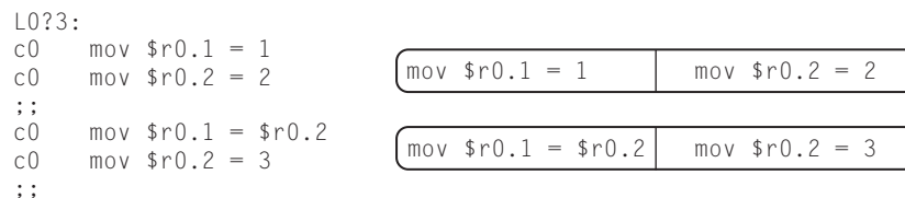
FIGURE 3.1 A contrived code example, the operations that make up the instructions for the example, and different possible horizontal semantics within an instruction. If a read sees original values, $r0.1 will have value 2 after these instructions execute. If a read sees the values of a parallel write, $r0.1 will have value 3 after these instructions execute. The second instruction is illegal for VLIW architectures that prohibit reading and writing the same register in a single instruction.
