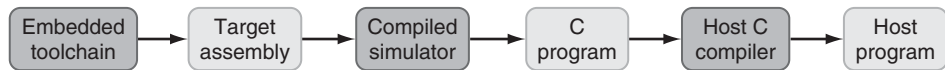
FIGURE 6.11 How compiled simulation works. This workflow diagram shows an embedded toolchain producing a “target program,” which is translated by the compiled simulator to the “C program,” which is compiled by the host’s native C compiler into the “host program.” We then run the host program on the actual data for the simulation.
