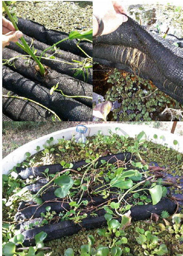
Fig. 3 Floating island prototype built with plastic fabric, PET bottles, and wood shavings as filler, vegetated with E. grandiflorus , H. ranunculoides , S. montevidensis , and P. rotundifolia . Prototype design: Gabriel Basflico
