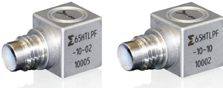
Fig. 9.9 Photographs of the designed 175 °C, 10 mV/g triaxial IEPE accelerometers comprising 2-pole active LPF and having size of 10 mm 3
