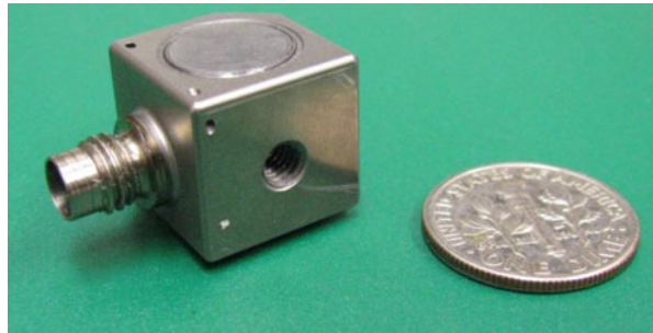
Fig. 9.3 Photograph of the designed 175 °C, 100 mV/g triaxial IEPE accelerometer
