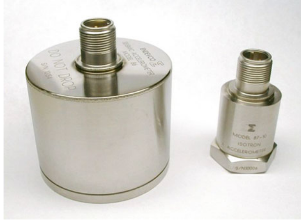
Fig. 8.3 Photograph of the designed accelerometers
