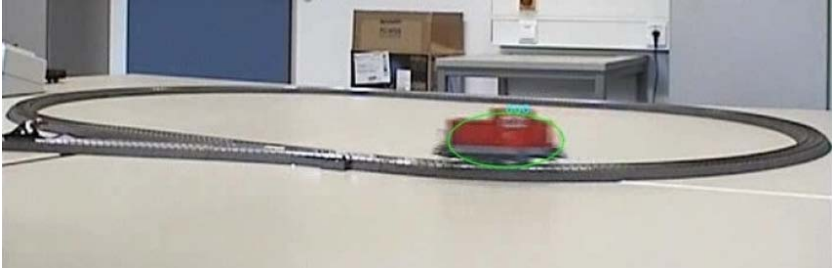
Fig. 4. Laboratory testbed: model railway tracked by Smart Camera (indicated by an ellipse)
