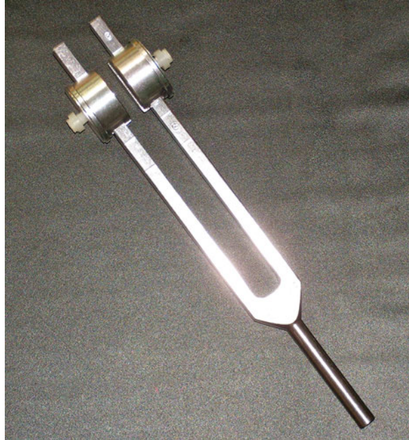
Fig. 5.3 A tuning fork with adjustable weights to tune the frequency (photo by the author)
