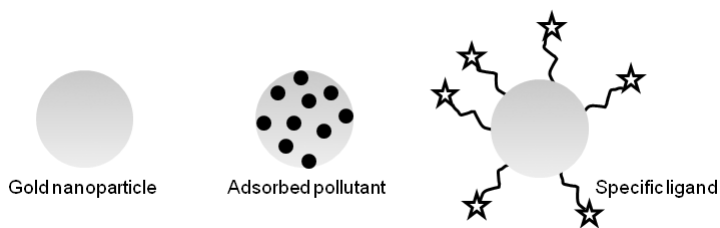
Figure 17.1 Surface modification of a AuNPs, either by adsorption of a pollutant, or by functionalisation with a ligand, specific for a chosen cell membrane transporter.
