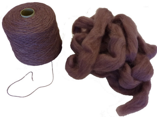
Figure 18.5 High-quality wool that has been dyed purple using AuNPs that have been grown in situ on the fibre. Photo courtesy of Prof. J. Johnston, Victoria University, New Zealand. Further detail may be found in Ref. 45.
