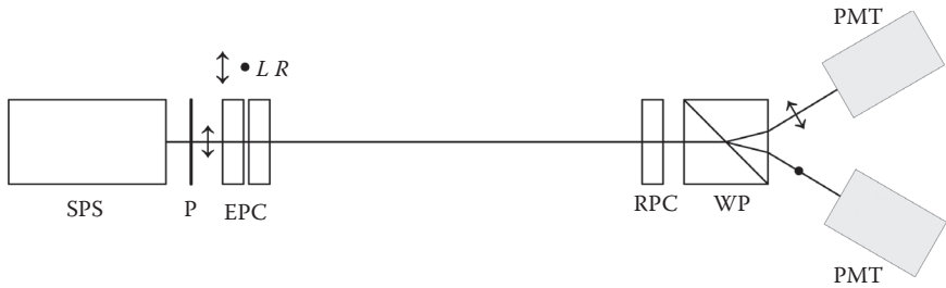
FIGURE 19.5 Top view of a generic experimental configuration applicable to the Bennett–Brassard protocol. The emission from a single-photon source (SPS) is linearly polarized by a polarizer (P). Then follows a polarization control system usually comprised of the EPC (see text). These are phase shifters used to select \leftrightarrow , \updownarrow , L , or R polarization states. Following propagation the photon reaches the RPC prior to being discriminated by a WP. For a description of the WP, refer to Chapter 15.
