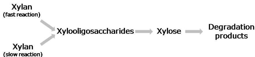
Figure 3. Xylan acid hydrolysis and possible steps. A complex scheme should be developed considering the recalcitrance and material heterogeneity. The xylan can be at different degrees: soluble, acetyl content, branches, accessible and lignin protected.
