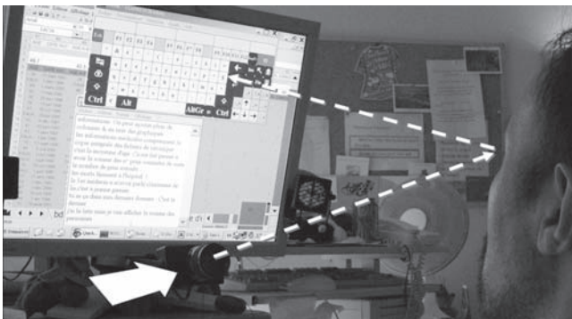
FIGURE 15.3 A locked-in person updates the database of ALIS, moving the cursor on screen by eye movements. An infrared camera (white arrow) mounted below the monitor observes one of the user’s eyes, an image processing software continually analyzes the video image of the eye and determines where the user is looking on the screen. The user looks at a virtual keyboard that is displayed on the monitor and uses his eye as a computer-mouse. To ‘click’ he looks at the key for a specified period of time (typically a fraction of a second) or blinks. An array of menu keys allow the user to control his environment, use a speech synthesizer, browse the worldwide web or send e-mail independently (picture used with kind permission from DT). With a similar device Philippe Vigand, locked-in since 1990, has written a testimony of his LIS experience in an astonishing book ‘Putain de silence’ translated as ‘Only the eyes say yes’ [48].
