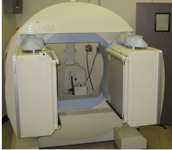
Fig. 20.1 Image of a dual-head clinical gamma camera
