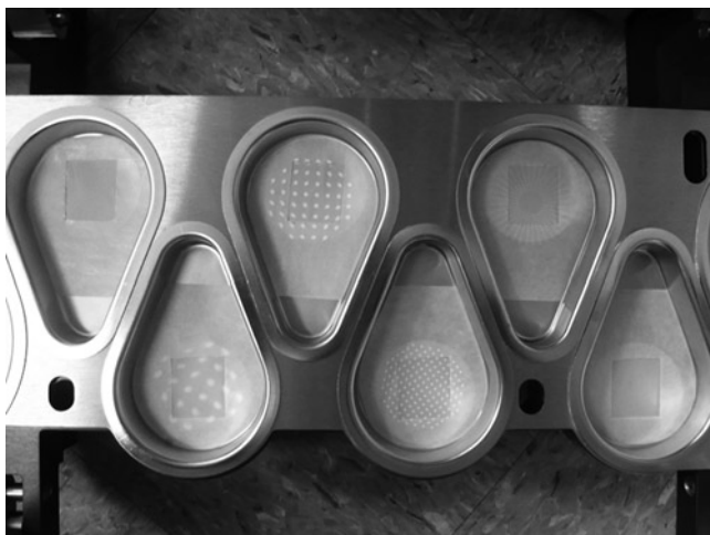
Fig. 17.20 Aerodynamic separation into the modified next generation impactor (NGI) for dose collection (from Son and McConville [82] with permission)
