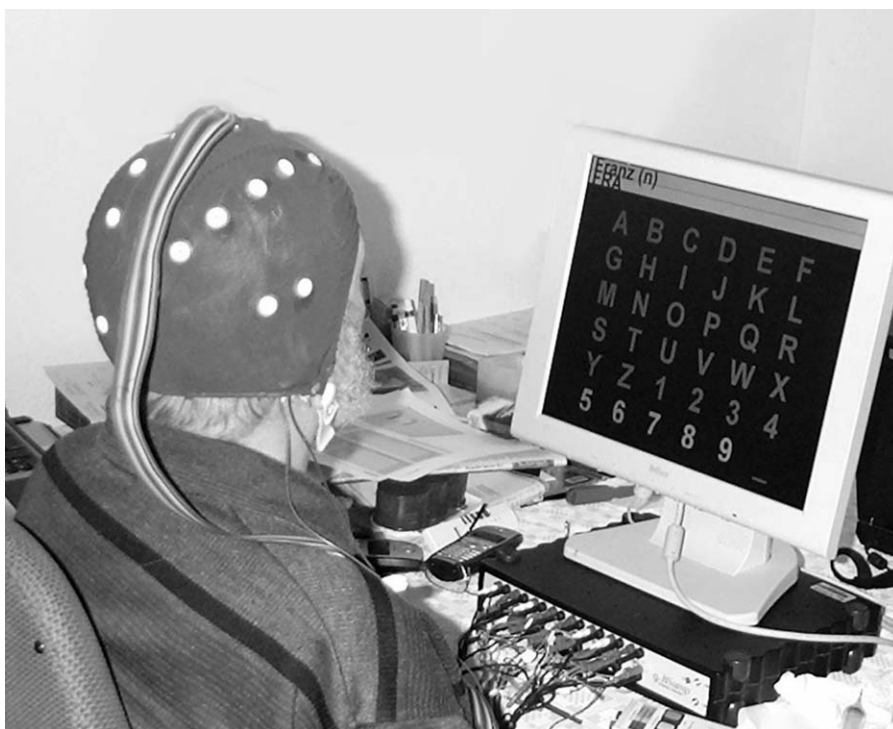
Fig. 3. A patient during training with the P300 BCI. The patient is trained at home under the supervision of an assistant from the laboratory. He views a 6 \times 6 letter matrix and is required to copy the word on the top of the screen (Franz). He has already copied correctly FRA and is now counting how often the letter N flashes (for details about the method see section on “event related potentials”).
