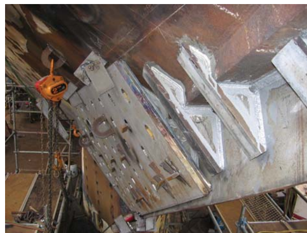
Figure 10: Fitting the warped side plates
