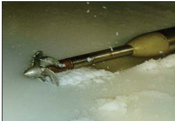
Figure 4: Propeller model test for ice milling mode in ice tank of Krylov Shipbuilding Research Institute
