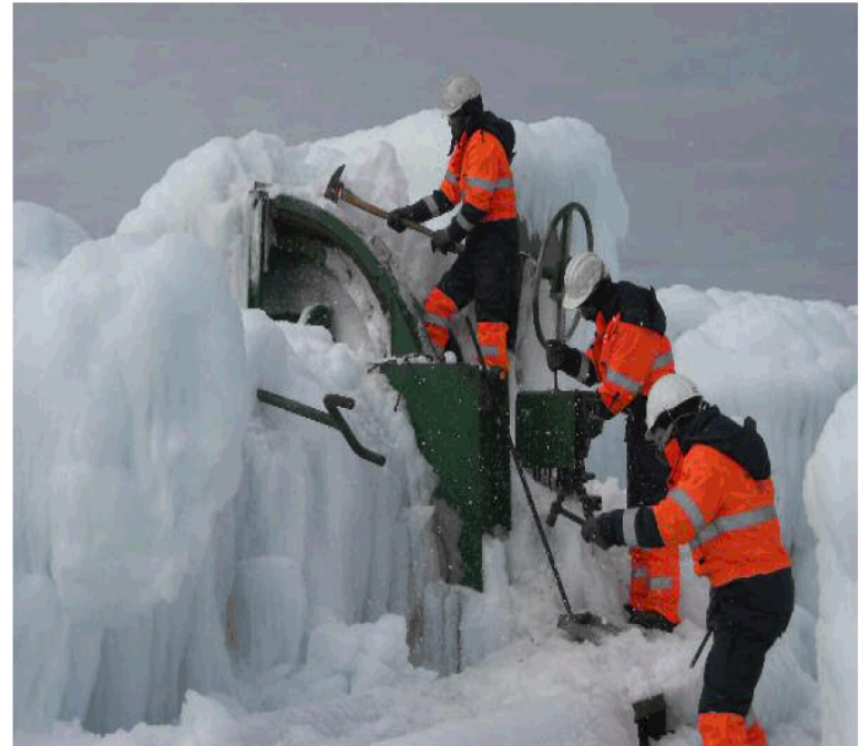
Crewmembers of a BP Tanker seen clearing the "Frozen Spray" from the anchor windlass
