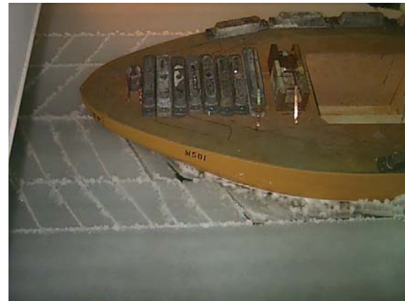
Figure 2: Model Tanker In Pre-Sawn Ice
