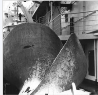
Icebreaker propeller blade failure along "skewed" peripheral blade section
