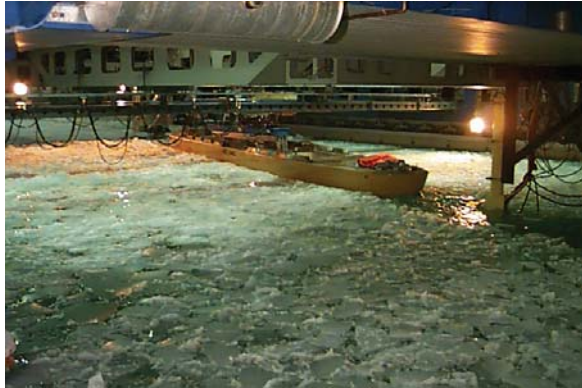
Figure 3: Model Tanker In Pack Ice, 95% Concentration
