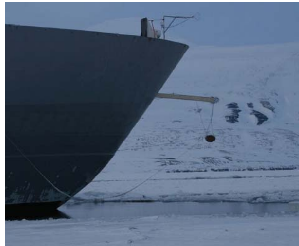
Figure 5: EM device mounted in the bow of KV "SVALBARD"
