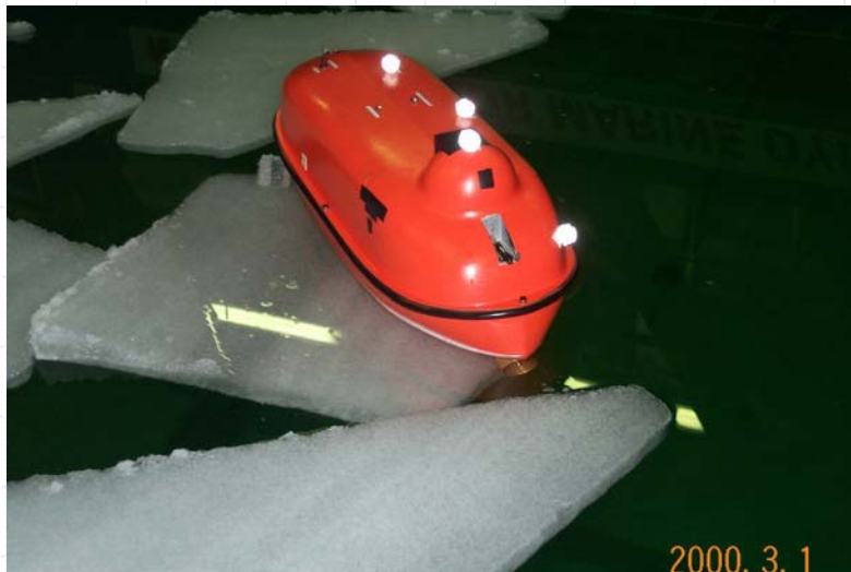
Ice Tank with model lifeboat
