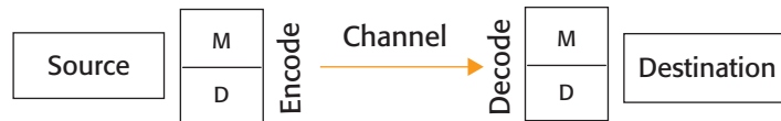
Figure 22.10 Once data (D) have been encrypted according to a code, they can be securely transported across a communication channel like the Internet. To be able to decode the data, one must possess a key or code that is the model (M) used to encrypt the data.
