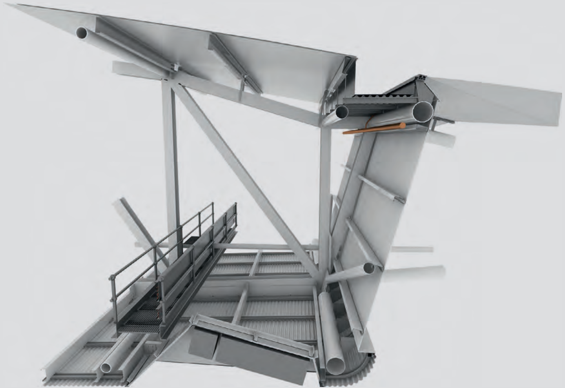
Figure 1-2 Detailed facade systems generated via BIM and visualized as a 3D rendering by COX Architects.
