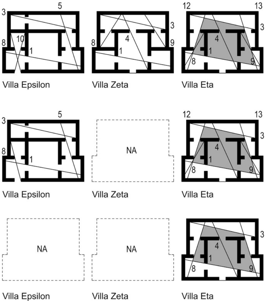
Fig. 3.22 Iterations five, six and seven of Step 9; the complete set of lines for the three villas are tested and, following the protocol, lines are removed until only an optimal set remains for each plan. (NA = not applicable, because some plans require repetition of various steps while others do not)
