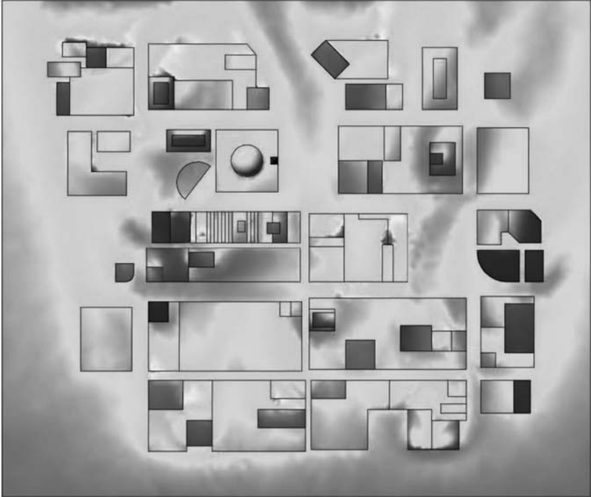
Figure 14.8 CFD-derived temperature effects at ground level.
