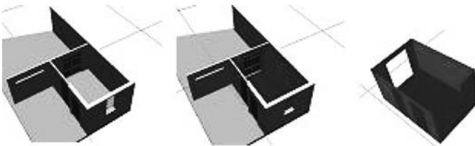
Figure 7.18 Automatic 'builder' adding finishes to the BIM.
