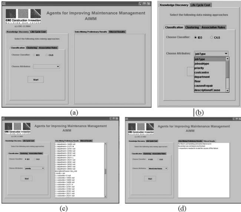
Figure 21.6 (a) The AIMM prototype system is instantiated once a building asset type has been selected; (b) data-mining techniques and different attributes for the user to choose from based on focus and interest; (c) preliminary results of applying the ID3 with the ‘Priority’ attribute on the maintenance data of Air Handling Unit; and (d) an example of the filtered knowledge presented to the user from the preliminary results of applying the ID3 with the ‘Work Order Status’ attribute on the maintenance data of Air Handling Unit.
