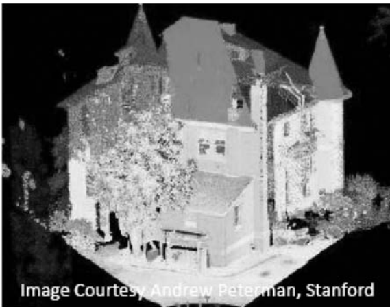
Figure 16.3 Point cloud-defined using laser scanning (source: Andrew Peterman, Stanford University).
