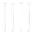
Nails DIN 1151 wire nails DIN 1143 machine nails
