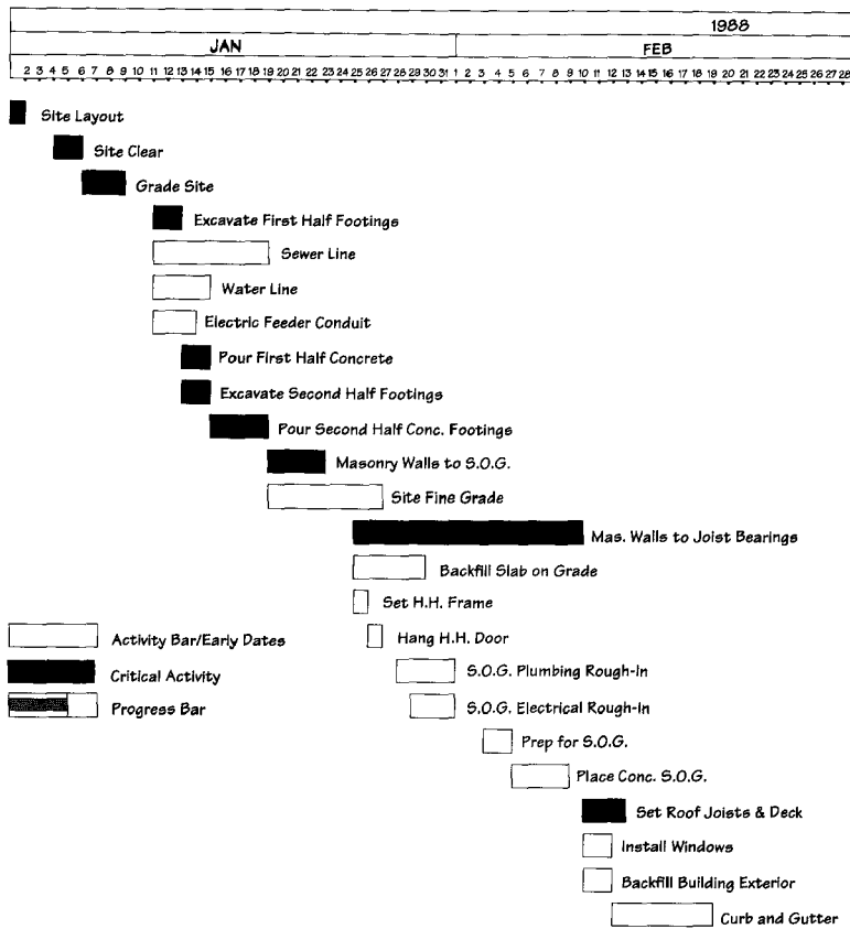
Figure 130-4. A project bar diagram based upon a PERT diagram showing beginning and ending times of all tasks. The critical path is shaded.
