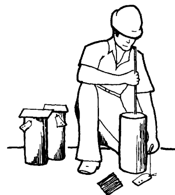
Figure 830-2. Cylinder test (ASTM C31). Cardboard or steel molds are filled with fresh concrete in three equal layers, and each layer is rodded 25 times with a 5/8-in.-diameter tamping rod. Cylinders are leveled and covered with a plate or plastic bag.
