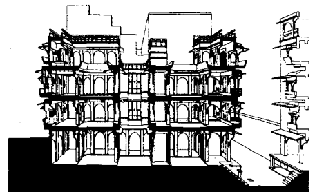
Fig. 34: Exploiting the stack effect: fresh air flows through the open ground floor and rises in the internal courtyard. House, Jaisalmer (India), 15th century
