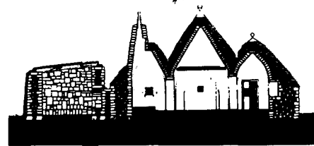
Fig. 28: Multi-leaf wall with filling of loose, low-quality material (section) Trulli – traditional solid stone buildings of southern Italy, Sovero (I)
