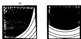
Fig. 8: Distortion of squared sections during drying
