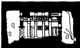
Fig. 23: A Lalibela Church, Ethiopia, c. 1400 The rock has been worked on all sides to create monolithic walls and columns.
