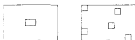
Fig. 7: Grouping versus decentralisation Schemes with stove and bathroom combined in the centre of the house (left: short service lines), and a decentralised layout (right: many service lines)
