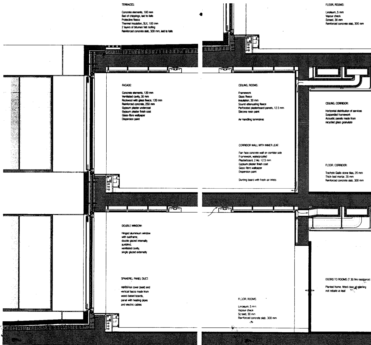
Fig. 197: Section through seminar room and corridor Services are routed in ducts along the spandrel panels and above the suspended ceiling over the corridor.
