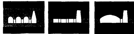
Fig. 21: Creating open space in solid rock Left: soft rock – short spans with arches Centre: hard rock – short spans without arches Right: hard rock – large span with arch
