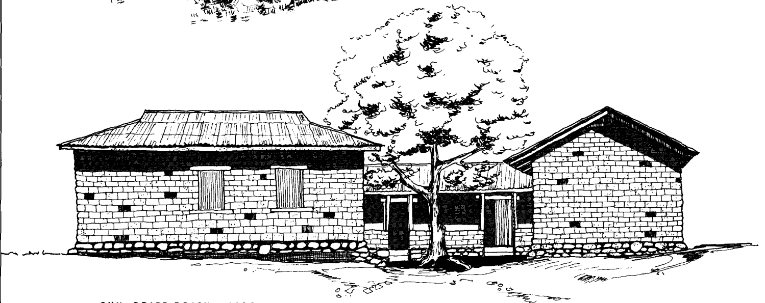
FIG.60 : SUN-DRIED BRICK WALLS , COMPOUND IN AVENYA, VOLTA REGION
