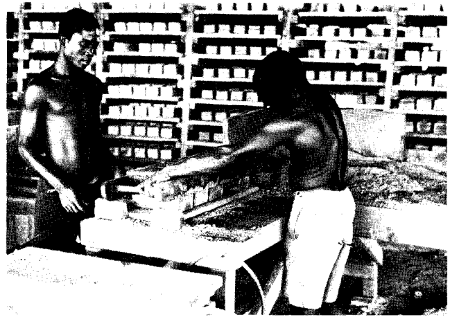
Fig. 142: ...removing bricks from mould onto drying board. Note drying racks in the background.
