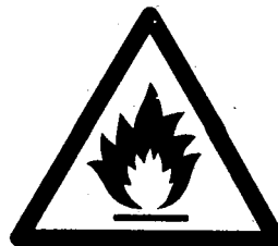
Risk of fire
