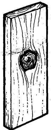
4 Board containing a dead knot
