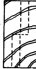
The effect of alternating the material face against the fence with off-centre mortises
