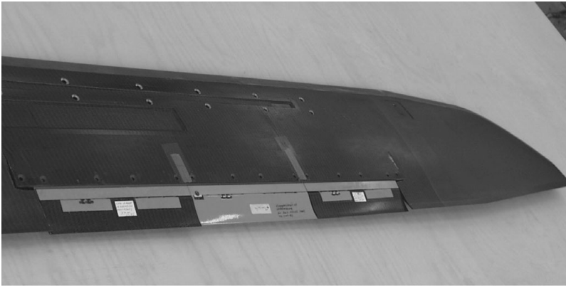
Figure 8.66. Full-scale BK117 rotor blade with trailing edge flaps and piezoactuators, from Ref. [155].
