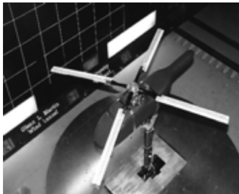
Figure 1.32. Active twist blade with embedded piezo actuators (6 ft diameter) rotor test in Glenn L. Martin wind tunnel; produced \pm 0.5 deg blade twist up to 5/rev excitation, from Ref. [205].
