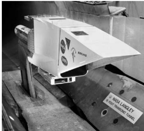
Figure 1.27. F-15 engine inlet used in the SAMPSON project, from Ref. [176].
