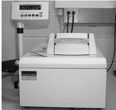
Figure 3.26. Differential Scanning Calorimeter.
