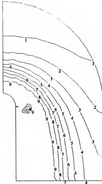
Figure 5, a) Case 2. Von Mises stresses for the adaptation; b) Case 3. Von Mises stresses for the ultimate state.
