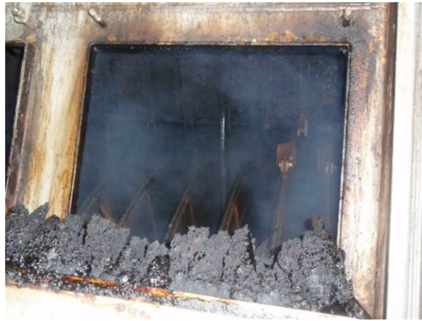
Figure 3. View into a disc dryer (picture by Author, 2011)
