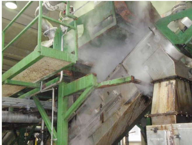
Figure 2. Top end of the coagulator with the press beneath (picture by author, 2011)
