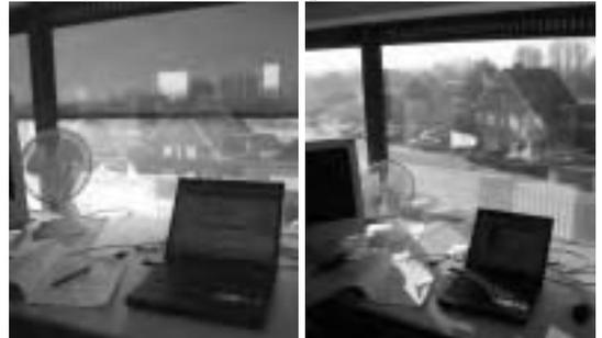
Figure 3: Impact of wind on functionality of external shading system. Left: Comfortable work space. Blinds are down due to intense solar radiation. Right: Blinds are up due to high wind speeds resulting in discomfort and overheating.
