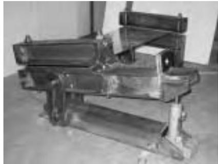
Figure 2: Test set-up for torsional tests
