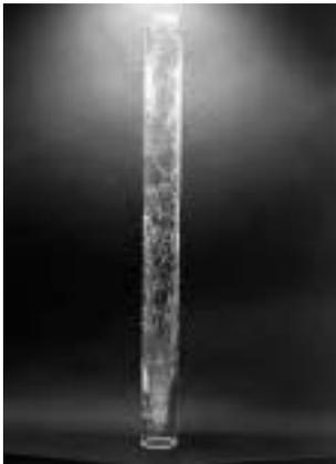
Figure 8: Glass compression test: fully broken inner tube still takes 110kN of compression force
