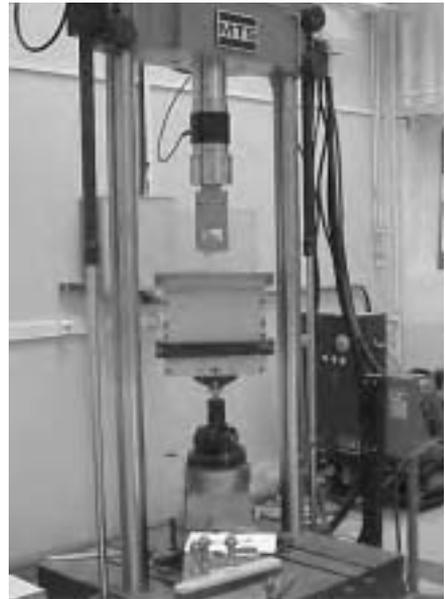
Figure 4: Failure test of a joint
