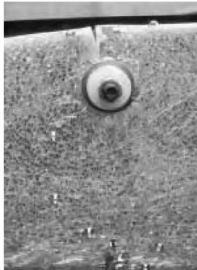
Figure 4: Stress concentrations around hole
