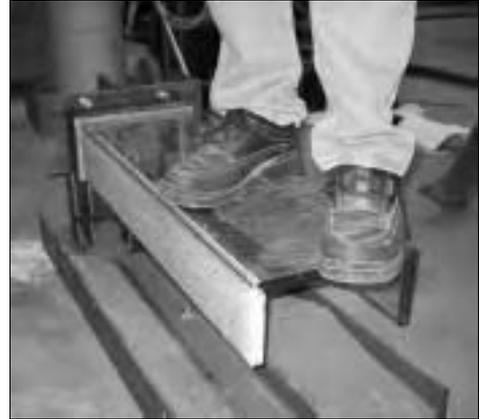
Figure 10: Both panels of one flange broken, tread still carries one person
