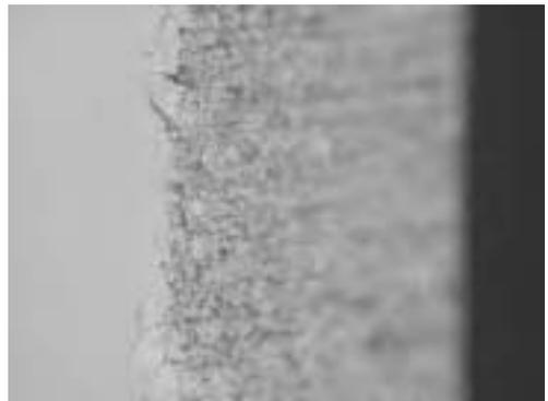
Figure 5: Arrissed edge of the annealed float glass
