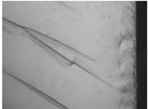
Figure 4: Cut edge of the annealed float glass
