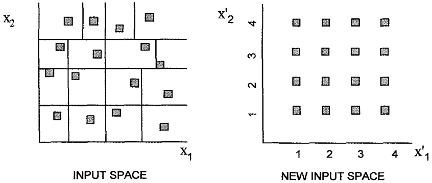
Figure 4.15: Data points can be mapped bijectively on a regular grid. Once mapped on a regular grid, the fuzzy-wavelet methods can be applied.
