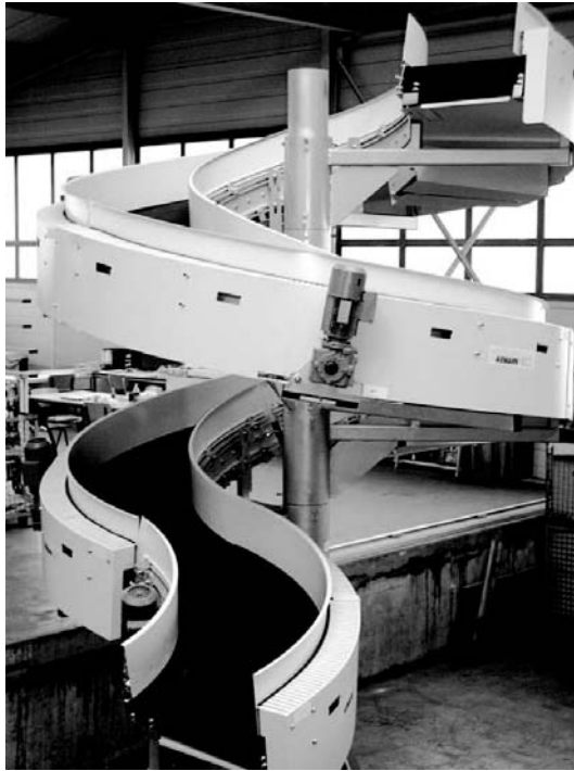
Figure 4.12. Conveying belt: Helical curve [Photo: AXMANN]
