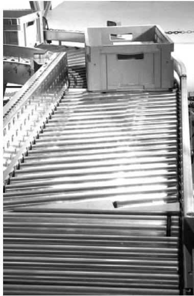
Figure 4.11. Roller conveyor. In the inlet the rolls are tilted to adjust the goods as shown on the right side of the picture. [Photo: SIEMENS DEMATIC]
