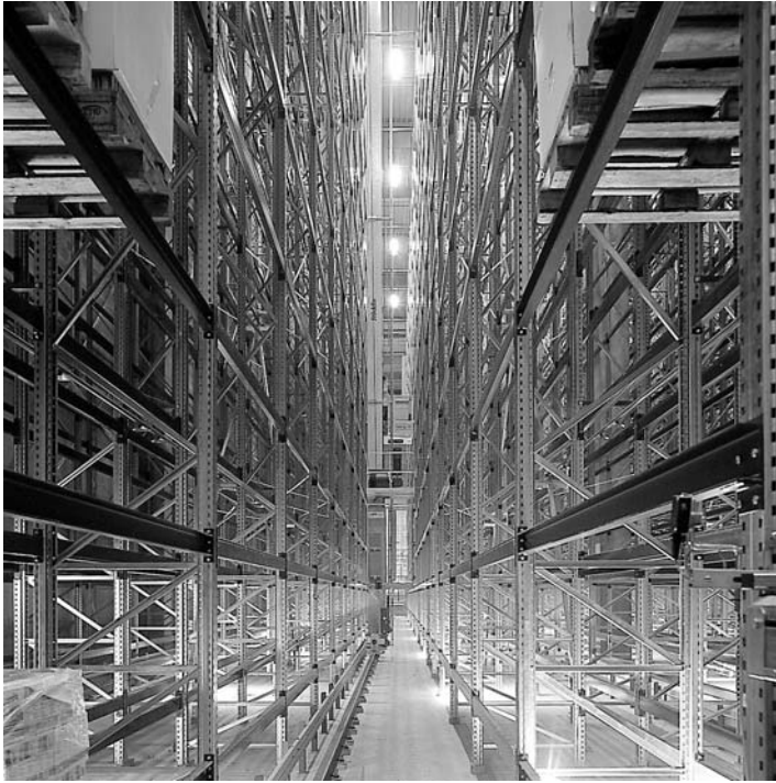
Figure 4.2. Pallet rack with lengthwise storage [Photo: STÖCKLIN SIEMAG]
