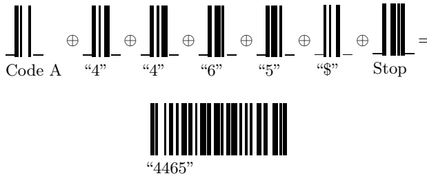
Figure 6.11. Digits “4465” with check digit in code 128 code A
