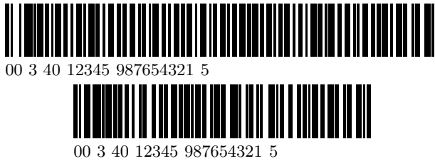
Figure 6.19. Comparison of the lengths of code A and code C with same contents
