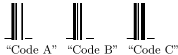
Figure 6.10. Start symbols for code A, code B and code C of the code 128
