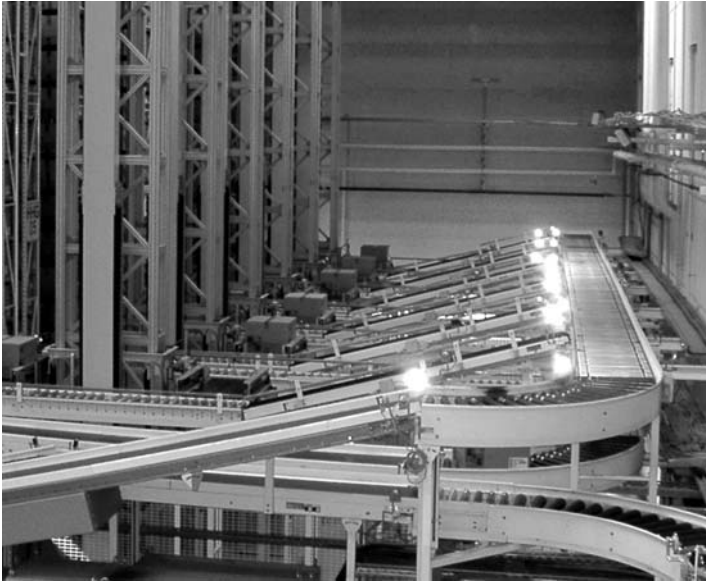
Figure 4.10. Pre-rack zone with conveyor. To avoid a clashing of incoming and outgoing flows the conveyor routes are arranged separately and on different levels to save space. [Photo: KHT]
