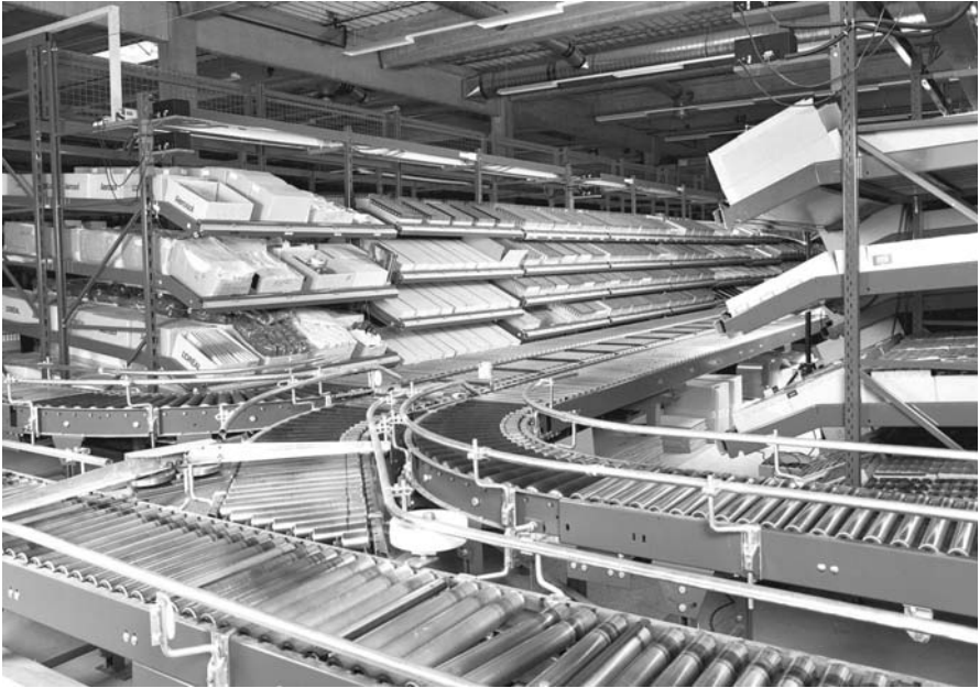
Figure 4.9. Flow rack with roller conveyors for order-picking according to the pick-to-belt principle [Photo: BITO]
