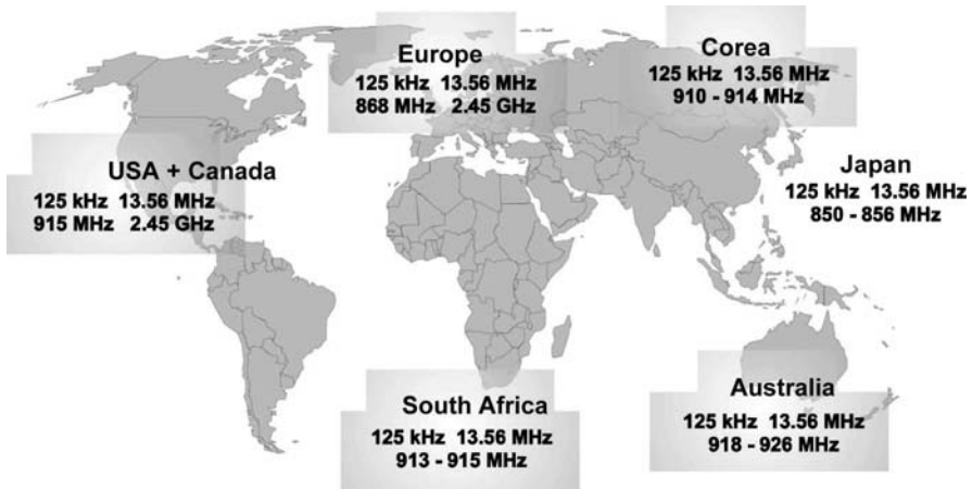
Figure 6.31. Frequency ranges for RFID systems (worldwide)
