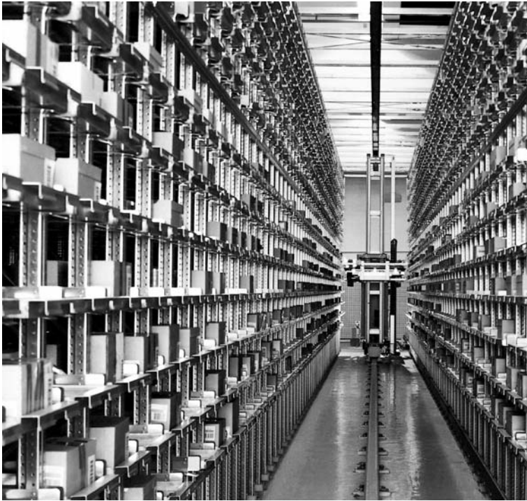
Figure 4.3. Automatic mini-load system with trays [Photo: BITO]
