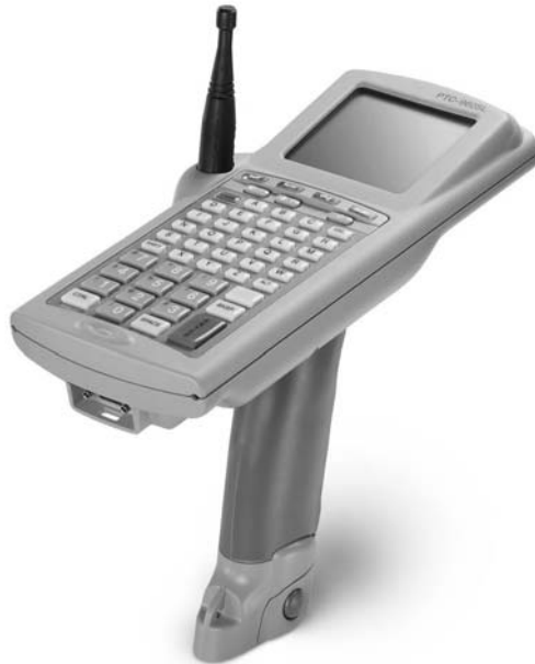
Figure 7.15. Typical terminals with barcode scanner, text display, keyboard and radio data transmission [Photo: SYMBOL]
