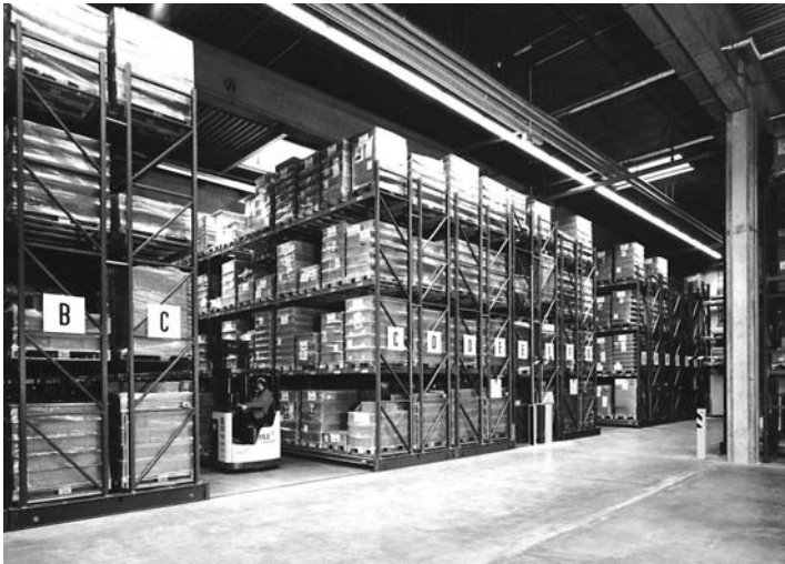
Figure 4.7. Movable aisle systems [Photo: META]
