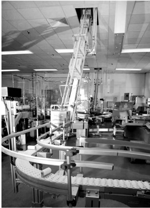
Figure 4.13. Chain conveyor: Flexible link conveyor for light piece goods (Carrying chain conveyor) [Photo: FLEXLINK]
