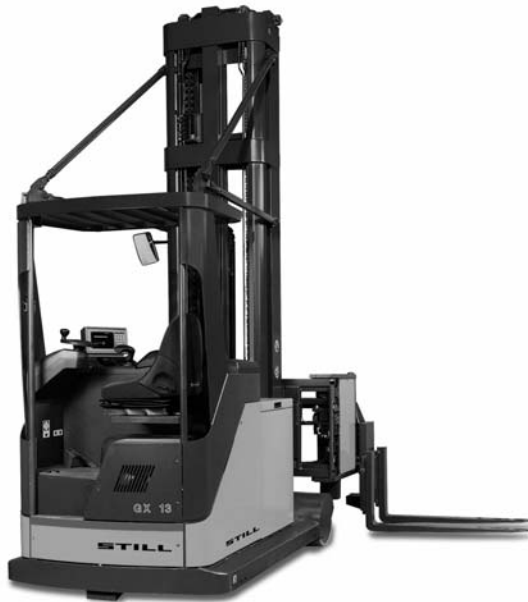
Figure 4.20. High-bay stacker with swivel fork lift [Photo: STILL]
