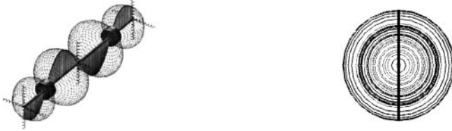
Figure 1. A whirling mode shape (natural frequency at 242 Hz) of a rotating rotor (at 1200 Rev./min.) having isotropic supports. The thick line indicates the location of the shaft centre at t=0 . Left – Animated response, Right- front view of the modeshape
