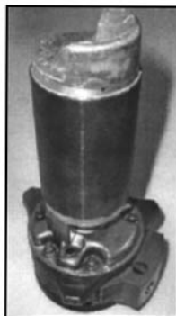
Figure 1: Motor compressor set
