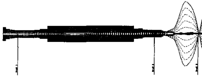
Figure 6 - Exciter-Generator Critical Speed at 1,454 RPM (24.2 Hz)
