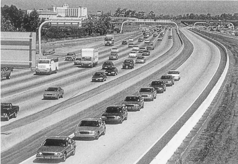
Figure 5-2. Platoon of Buicks used in the NAHSC Demonstration
