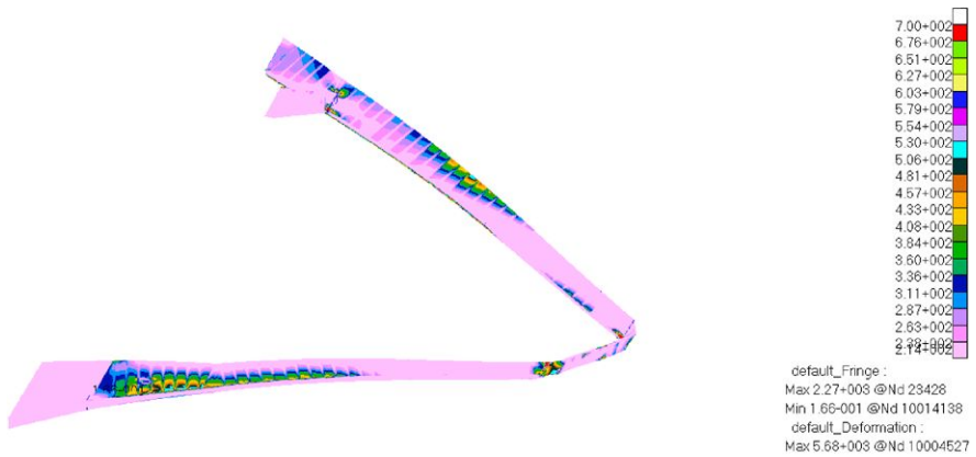
Fig. 7 Von Mises’s stress for the asymmetrical wing box in the step B case—bottom isometric view
