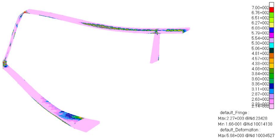
Fig. 6 Von Mises’s stress for the asymmetrical wing box in the step B case—top isometric view
