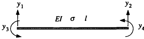
Fig. 8.6 Finite element model of a uniform free-free beam with one element.
