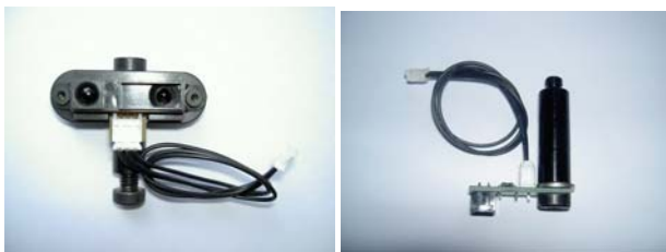
Fig. 5. Left: Bearing Sharp IR distance sensor. Right: Bearing for a CNY70 line sensor.
