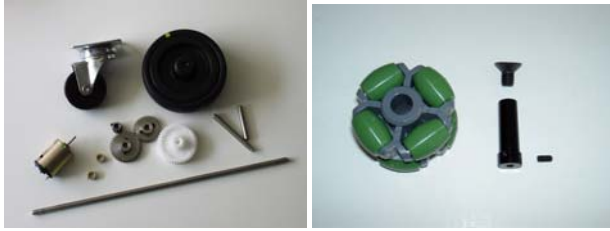
Fig. 3. Left: Wheels, axles and gears. Right: Omni wheel with its axle.
