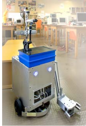
Fig. 3. RH3-Y, our mobile, cooperating robot for demonstrations in domestic applications. Blue trays, with individual covers, are there for user purpose, in « at home » applications. The lower level contains electrical and electronic devices, servo controller and PLC ;. the supervision computer can be lying on top of the trays, for development phases, but is normally smaller and also confined in the lower part of the robot; or is replaced by a fixed, regular computer, operating remotely via Ethernet and TCP/IP connection.
