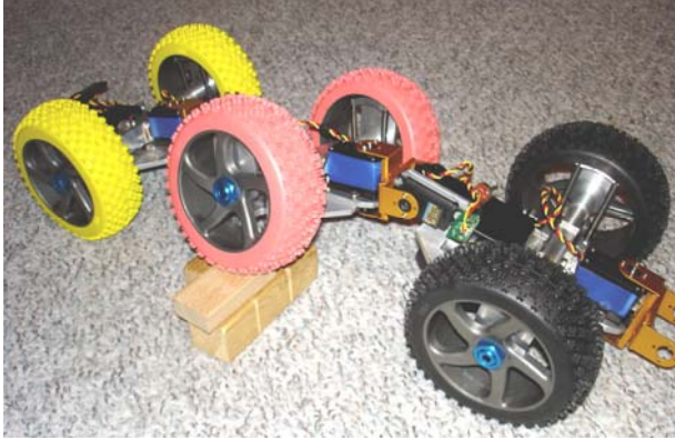
Fig. 7. Prototype of Wheeler on an uneven terrain – 3 segments (out of planned 7 segments) connected with 2 DOF joints
