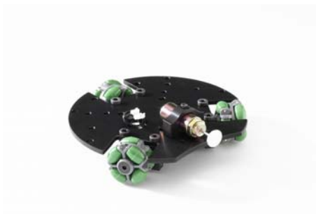
Fig. 12. Omnidrive platform with three omnidirectional wheels
