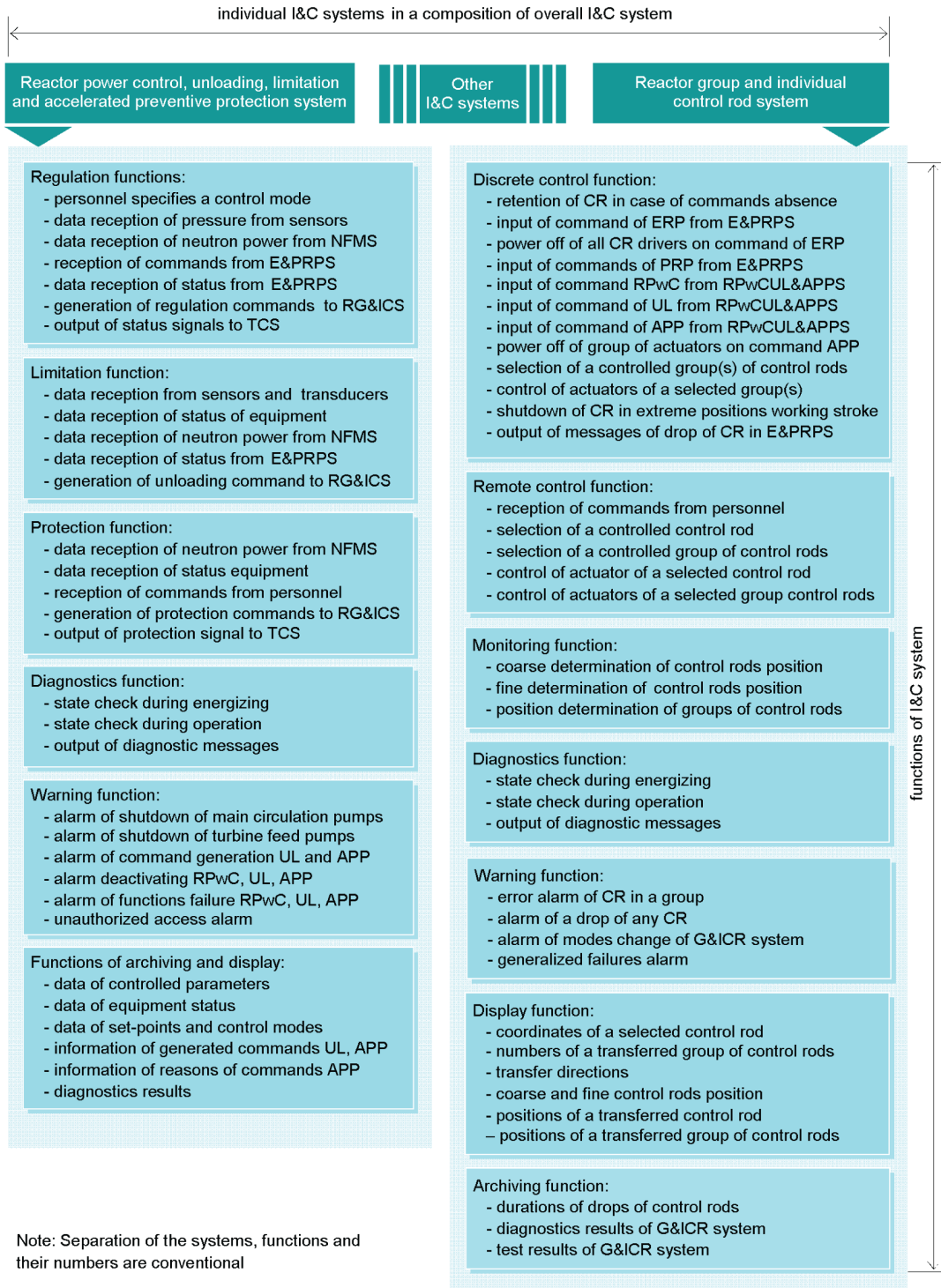
Figure 3. Functions of I&C systems: examples of a system point of view
