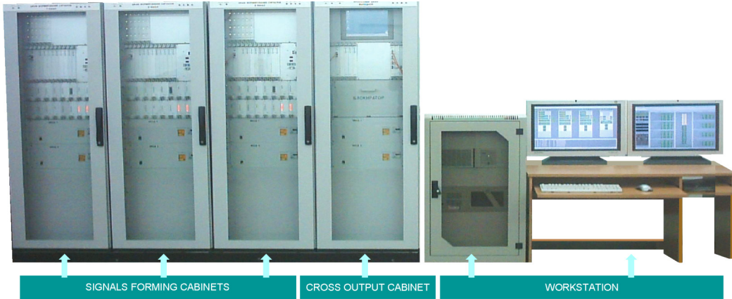
Figure 6. Software-hardware complex SHC E&PRP: external appearance
