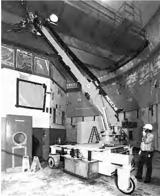
Fig. 1. The Rosie Mobile Worksystem at the CP-5 Reactor. (Courtesy of Sharon Curd at Oak Ridge National Labs)
