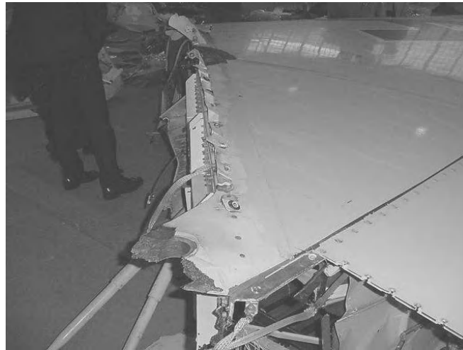
Figure 3.3. Service failure of a vertical tail at several fitting points
