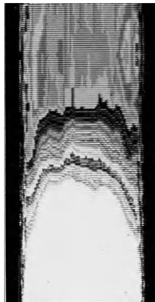
Figure 3.8c. Delamination of composites; tomographic radiography of the delamination and the damaged zone within its core
