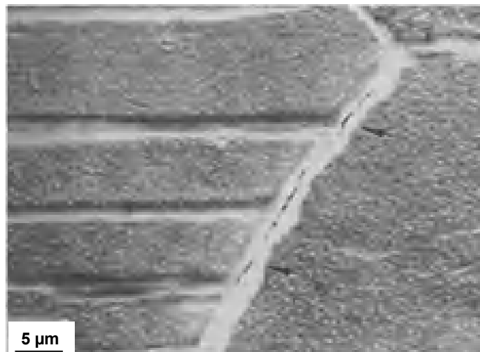
Figure 1.59. Slip-band-induced cracking of oxidized grain boundaries in Waspaloy tested in LCF at 527°C. Microcracks are indicated by the dark arrows [LER 84]
