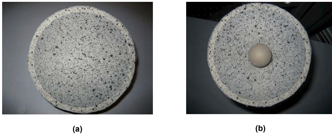
Fig. 2 (a) Latex membrane specimen attached with circular ring subject of the experiments (b) The painted steel sphere of weight 0.66 N placed at the center of the membrane for static test
