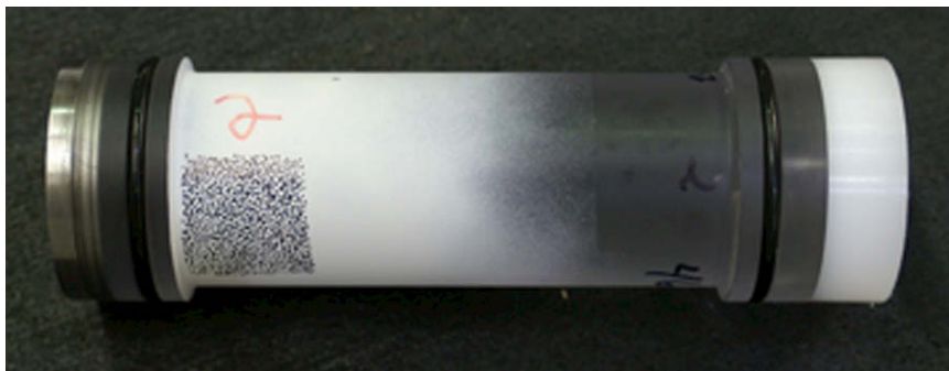
Figure 3. Image of the 50.8 mm diameter polycarbonate sabot assembly showing the AISI 4140 hardened steel anvil, polyethylene obturator and Viton ® o-rings.
