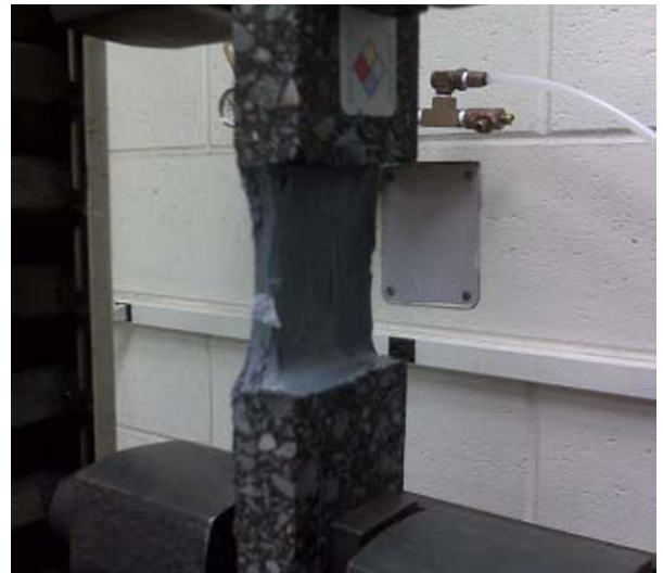
Figure 3. Testing Specimen Under Tensile Testing
