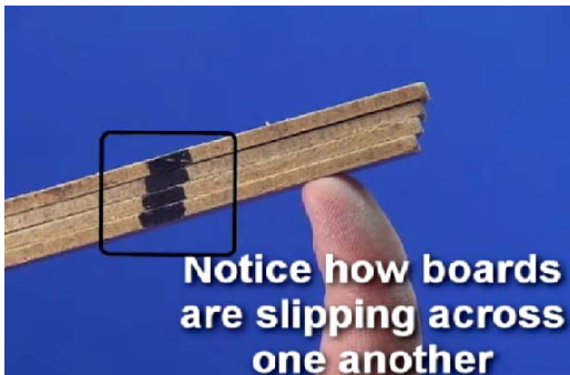
Figure 1: Use of text and box outline highlights an important aspect of this portion of the “Transverse Shear” demonstration.
