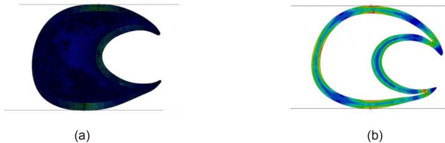
Figure 4: Finite element analysis results of (a) full petiole section and (b) skin section
