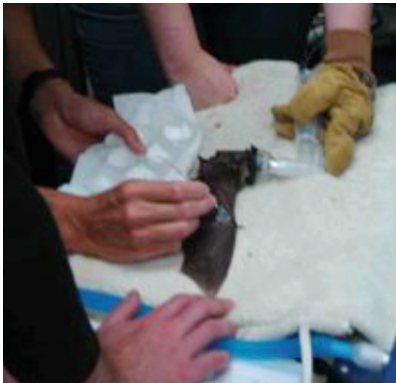
Figure 5. The anesthetized bat during the application of the speckle pattern on its right wing.
