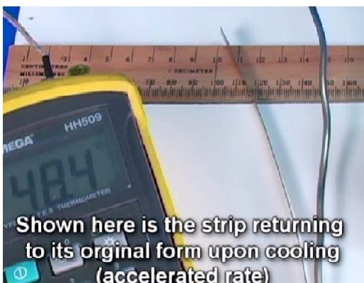
Figure 1: An image during data collection of temperature vs. deflection of the bimetallic strip is shown here.
