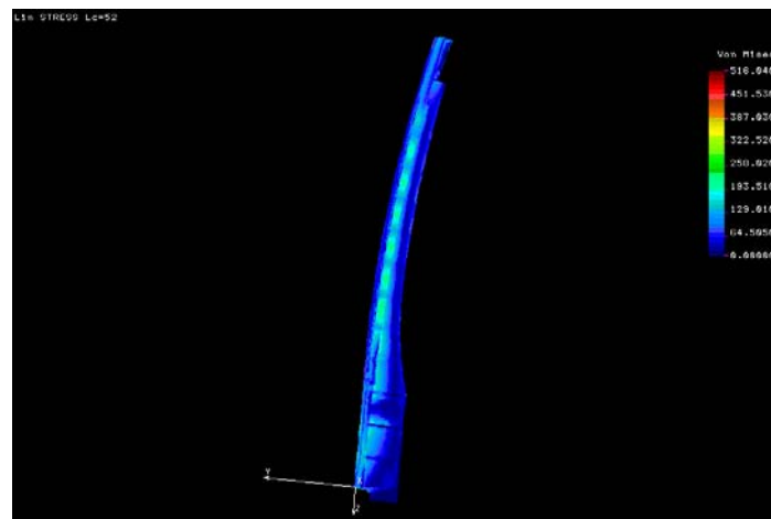
Fig. 5. Stress results of the third flap subjected to static loads
