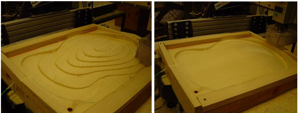
Figure 10 – Machining the Convex Side of the Plate
