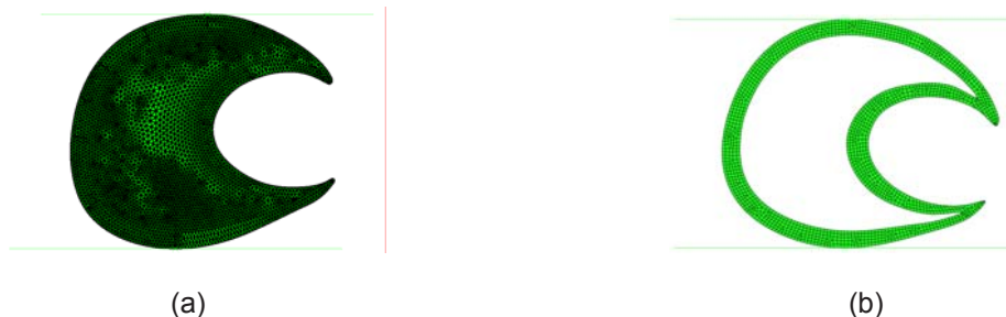
Figure 3: Finite element models of (a) full petiole section and (b) skin part of petiole
