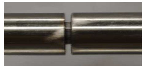
Figure 1: A Specimen Sandwiched between Incident and Transmission Bar
