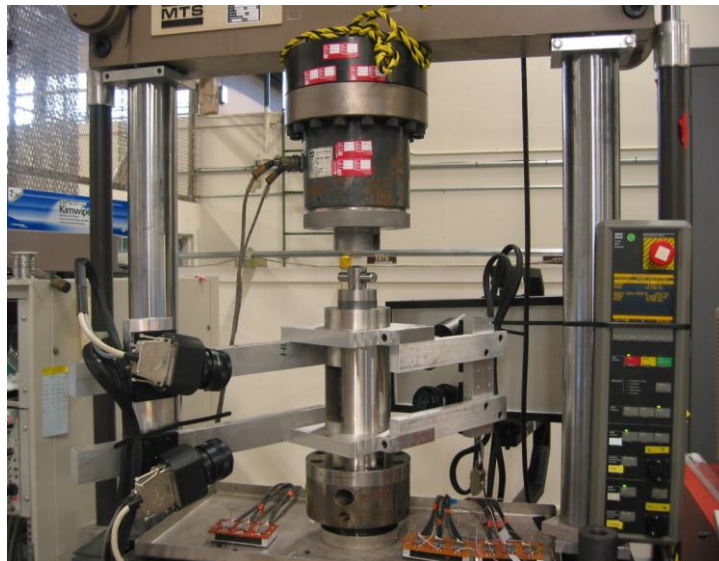
Figure 2 Test configuration for combined compressive and torsional loading.
