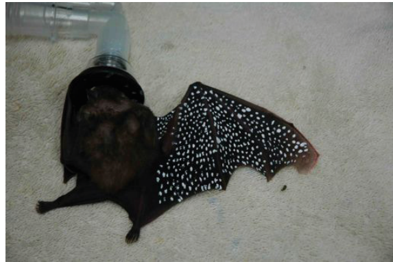
Figure 6. The bat's wing with the final speckle pattern.
