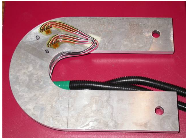
(b) Specimen side with rosettes B and D
