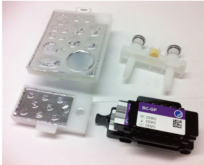
Fig. 2 The four consumables used for the Verigene BC-GP Test: Extraction Tray ( top left ), Tip Holder Assembly ( top right ), Utility Tray ( bottom left ), and BC-GP Test Cartridge ( lower right )
