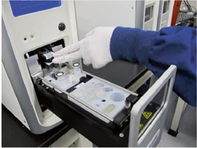
Fig. 6 User loading the consumable and BC-GP Test Cartridge into the Processor SP
