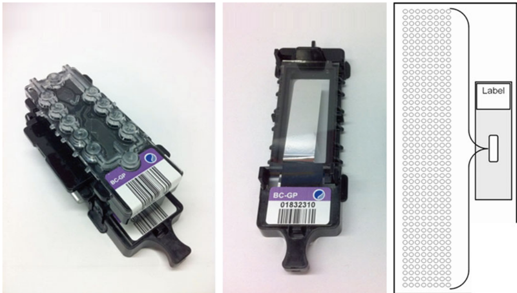
Fig. 3 The Verigene BC-GP Test Cartridge is composed of a Reagent Pack ( left ) and a Test Substrate ( middle ), composed of a microarray ( right ) spotted in the middle of the Test Substrate
