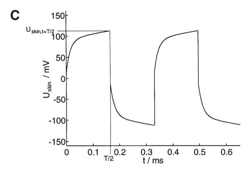
Fig. 4 (continued) and (C) the transdermal voltage  $[U_{skin}(t)]$  can be measured. These time domain measurements can be analyzed to yield values for the electrical circuit elements shown in **Fig. 3**.
