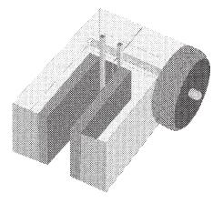
Fig. 1. Plate electrodes. Metal electrodes mounted on insulating material, with a screw that makes it possible to separate the two parts of the electrode for positioning. When the screw is tightened, the two plates of the electrode are held in parallel position. The distance between the plates is 4 mm, and the plates are 10 mm wide. The electric field distribution for these electrodes is reported in **ref.** 11.
