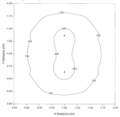
Fig. 6. Isoelectric field lines around a two-needle array. Field strength: V/cm; potential applied: 942 V; distance between needles: 0.65 cm.
