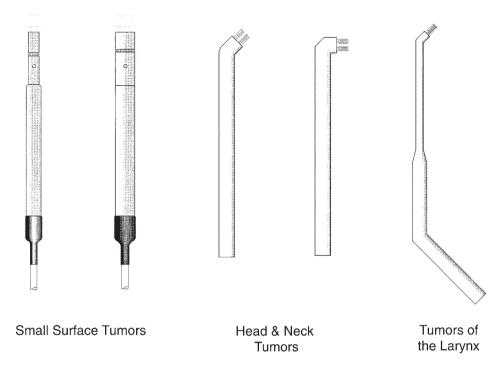
Fig. 11. Various six-needle array applicators.
