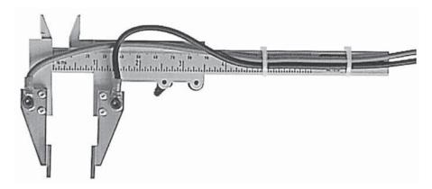
Fig. 4. Caliper electrodes for the treatment of subcutaneous tumors. The scale on the caliper allows measurement of the electrode distance so that the generator voltage can be set according to the desired field strength: E = V/distance.
