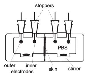
Fig. 5. Side-by-side permeation apparatus for clamping and bathing the skin specimen during electrical measurements. Four electrodes are held in place using Teflon stoppers as holders. The outer electrodes are used to apply electrical stimuli, while the inner electrodes are used only to make measurements. The skin is bathed on both sides by well-stirred saline. A water jacket surrounding the apparatus provides temperature control
