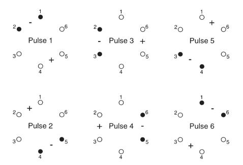
Fig. 8. Sequence used to energize individual needles for a six-needle array around the treatment site.
