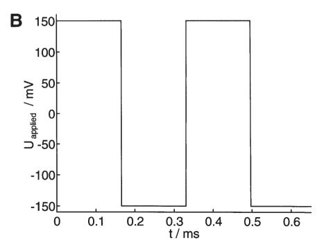
Fig. 4. Apparatus and representative signals for measuring skin electrical properties in the time domain. (A) The apparatus includes a measuring resistor  $(R_m)$  in series with a chamber containing skin. (B) A rectangular wave  $[U_{applied}(t)]$  is applied
