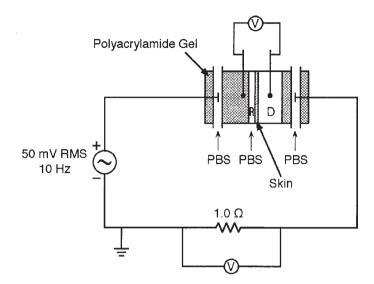
Fig. 6. Impedance measurement of the skin. The AC source produces a 50 mV RMS, 10 Hz bipolar sine wave. The current across the skin is determined by measuring the RMS voltage across the 1.0  $\Omega$  resistor placed in series with the skin. The voltage across the skin is measured with the voltmeter placed across the permeation chamber. The impedance of the skin is then found by Ohm's law.
