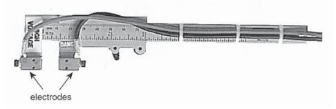
Fig. 2. Caliper electrode P/N 384 (Genetronics, Inc.) for in vivo transdermal drug or gene delivery. It consists of two brass electrodes that grasp the skinfold to be electroporated. The size of each electrode is  $1 \text{ cm} \times 1 \text{ cm}$ . The caliper scale allows accurate measurement of the distance between the electrodes.
