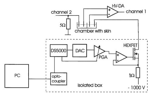
Fig. 14. Setup for the application of high-voltage signals of arbitrary wave form to skin. *See* text for explanation.
