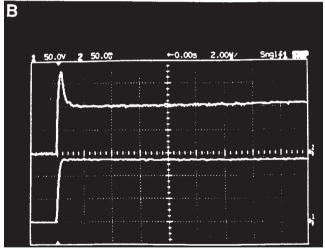
Fig. 6. Time track of the V(t) and I(t) curve during the pulsing monitored by a digital oscilloscope. In both panels A and B, the upper curve is I(t) and the lower curve is V(t). (A) Breakdown of the SC during the first pulse (120 V, 10 ms). (B) Breakdown of the SC during the third pulse (same as the first one). The resistance of the SC was decreased (I(t)) was increased compared with the first pulse) by electrical pore formation.
