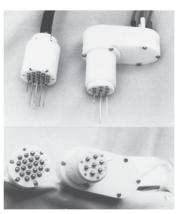
Fig. 1. Two examples of electrodes based on the principle reported in the text. **Right**: Template supporting seven parallel equidistant needles. **Left**: Template supporting nineteen parallel equidistant needles (the core of seven needles, as in the template shown above, surrounded by one more ring consisting of 12 parallel needles placed equidistantly to themselves and to the other needles in the inner array).
