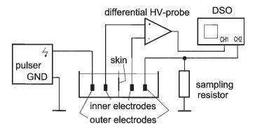
Fig. 8. Set-up for measuring the apparent resistance during a high voltage pulse. The pulser applies the voltage to the outer electrodes. A sampling resistor in series is used for current measurement ( $U_{sampling}$ ), recorded at the second channel (CH2) of the digital oscilloscope (DSO). To measure the voltage across the inner electrodes ( $U_{inner}$ ), a high voltage differential amplifier is used and  $U_{inner}$  recorded at channel 1 (CH1).
