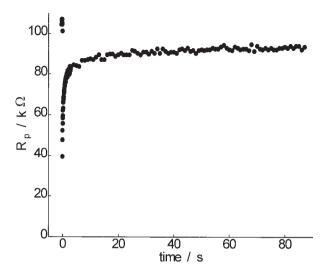
Fig. 9. Pre- and post-pulse impedance of human skin in vitro (A = 0.69 cm<sup>2</sup>). An exponential-decay pulse ( $\tau$  = 1.1 ms) was applied at t = 0 with an amplitude of 500V across the outer electrodes, which yielded a voltage across the skin of about 65 V. Since the DC-resistance ( $R_p$ ) is the most sensitive parameter it is the only one shown here.
