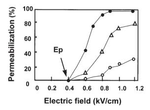
Fig. 2. Effect of the electric field parameters on the electropermeabilization of cells. CHO cells are pulsed at a 1-Hz frequency in the pulsation buffer in the presence of propidium iodide. The percentage of fluorescent cells is plotted as a function of the electric field intensity for different number of pulses and duration values: 10 pulses at 0.1 ms duration  $(\bigcirc)$ , 10 pulses at 5 ms  $(\triangle)$ , 20 pulses at 5 ms  $(\bullet)$ .
