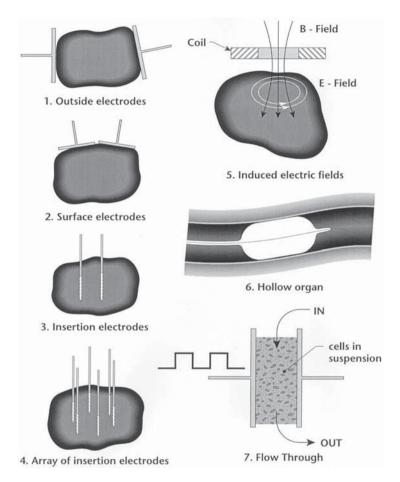
Fig. 2. Basic field applicator configurations.
