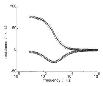
Fig. 1. Impedance spectrum of human stratum corneum in vitro  $(A_{skin} = 0.67 \text{ cm}^2)$  for a frequency range between 10 Hz and 1 MHz. Both the real  $(\times)$  and the imaginary  $(\bigcirc)$  parts of the impedance are represented.
