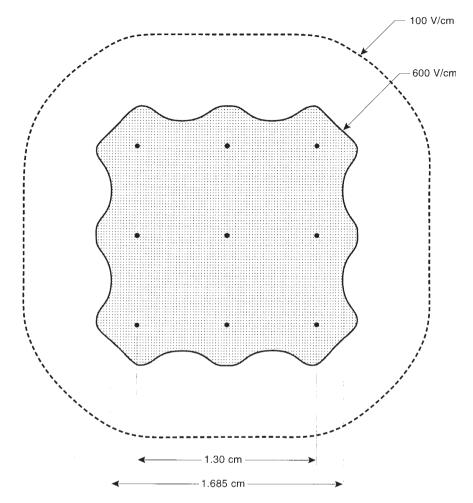
Fig. 13. Isoelectric field lines generated by array of four-needle squares after switching 90°; 0.65 cm base length; 940 V between needle pairs.
