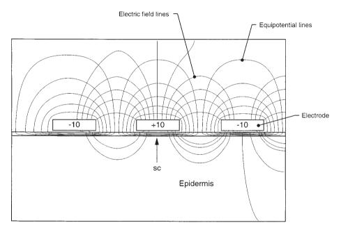
Fig. 16. Plot of equipotential and electrostatic field lines of meander electrodes on top of the SC with a distance of 10  $\mu$ m. Specific resistivities: medium surrounding the meander electrodes, 1000  $\Omega \times$  cm; SC,  $6 \times 10^8 \Omega \times$  cm; viable epidermis,  $10^5 \Omega \times$  cm. Potential difference between meander electrodes:  $\pm 10 \text{ V}$ .
