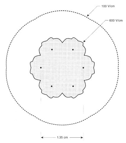
Fig. 10. Isoelectric field lines generated by a six-needle array (four are active), after switching 60°; 1.35 cm diameter; 1500 V between needle pairs.
