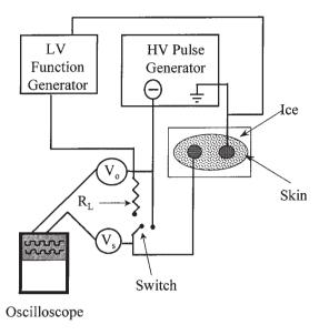
Fig. 1. Schematic diagram of electrical set-up. The low voltage function generator was used to measure the pre/post pulse resistance from oscilloscope measurements of  $V_{\rm o}$  and  $V_{\rm s}$ . The high voltage pulse generator was used to apply the permeating pulses and to measure the resistance during the pulse.
