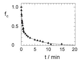
Fig. 1. Pore resealing kinetics indicated by dye uptake. The fraction  $f_{\rm C}$  of colored cells as a function of the time  $t=t_{\rm add}$  of dye addition after the pulse. B-lymphoma cells (line IIA1.6) were exposed to one rectangular electric field pulse (E=1.49 kV cm<sup>-1</sup>; pulse duration  $t_{\rm E}$  =110  $\mu$ s) in the presence of the dye SERVA blue G (M<sub>r</sub> = 854). (From **ref. 9**, with permission.)
