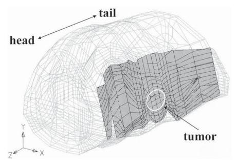
Fig. 1. Three-dimensional anatomically based finite element model of a mouse with subcutaneous solid tumor. Shaded plane represents cross section through the middle of the tumor in which the results were shown.
