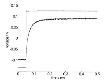
Fig. 7. Typical signal captured by the oscilloscope following electroporation of skin using the apparatus shown in **Fig. 6**. The step curve was recorded in channel 1 ( $U_{applied}$ ) and the deformed curve in channel 2 ( $U_{skin}$ ). The trigger appears at 0.05 ms. No averaging was used. The skin specimen was previously pulsed with  $U_{skin} \approx 55 \text{ V}$  and  $\tau = 1.1 \text{ ms}$ .
