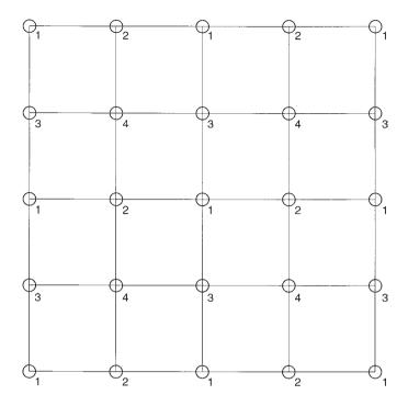
Fig. 14. Square needle array  $(2.6 \text{ cm} \times 2.6 \text{ cm})$  with paralleling all switching zones.
