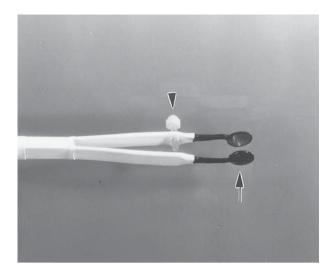
Fig. 1. Guilded stainless steel electrodes mounted on tweezers. The distance between the two electrodes (arrow) can be fixed by a plastic screw (arrowhead).
