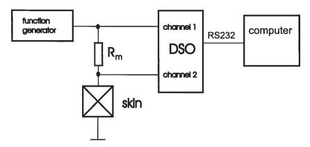
Fig. 6. A function generator provides a voltage across a measuring resistor ( $R_m$  is usually 10 k $\Omega$ ) and the skin chamber. For an applied voltage step the voltage across the skin will be deformed (e.g., as shown in **Fig. 4C** or **Fig. 7**) due to charging of capacitive structures in the skin.
