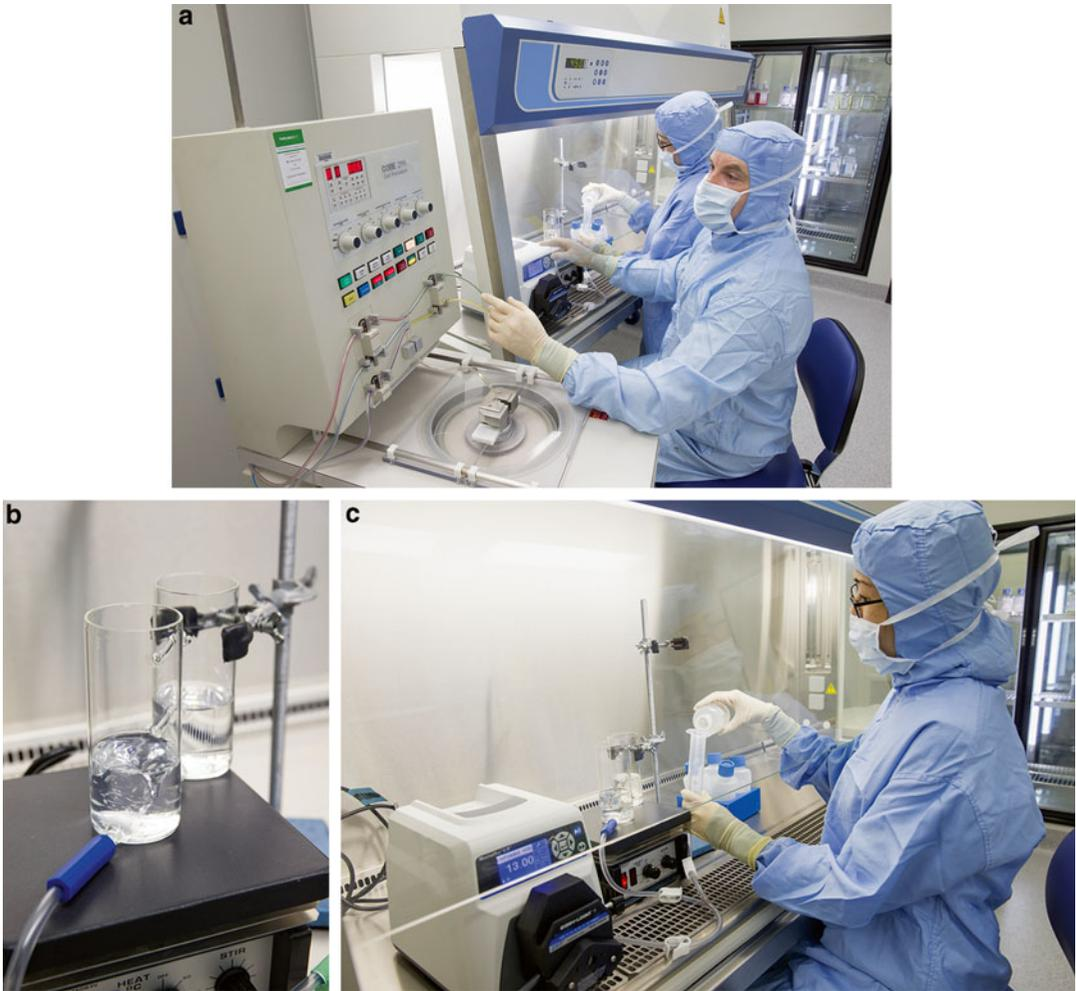
**Fig. 7.5** (a) Laboratory setup for the islet purification phase. In the foreground the COBE® 2991™ Cell Processor has been set up with a COBE bag that is being loaded with a continuous density gradient by a gradient mixer as shown in (b). (c) Shows top loading of the den-
