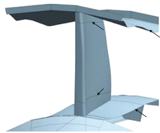
Fig. 3. A sector with some tagged welds indicated by arrows to be evaluated.
