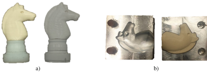
Fig. 7. Knight quality issues (a) Colour difference (b) Fixture for hole drilling.
