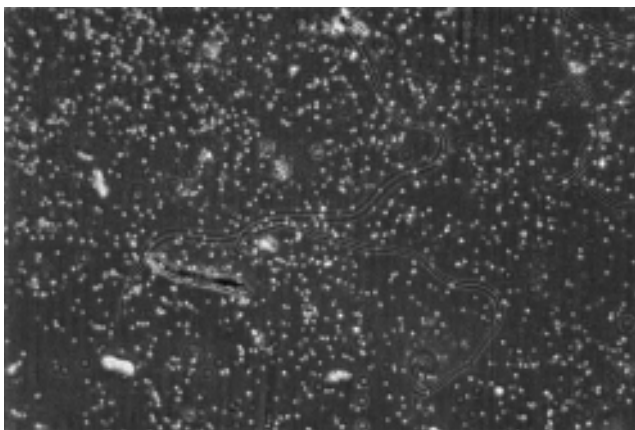
Figure 11.10 Excessive dispersed growth. Dispersed growth consists of small ( <10\mu\text{m} ) and spherical floc particles. In an “unhealthy” biomass the relative abundance of dispersed growth may be “excessive” or “hundreds” (100, 200, 300, ...) of small floc particles or “cells” per field of view at 100 \times total magnification.
