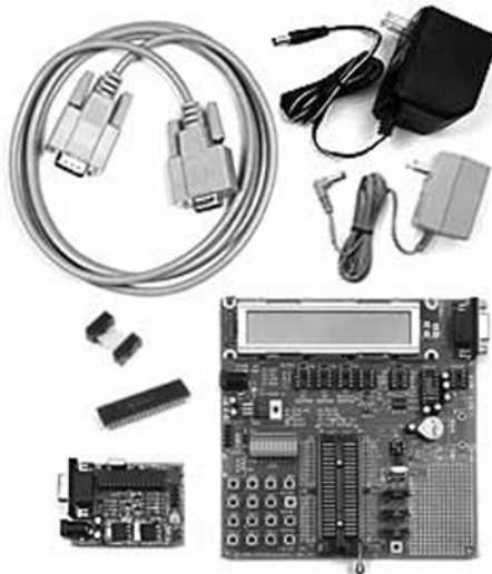
Fig. 3.31 LAB-X1 Bundle with serial programmer (Courtesy of microEngineering Labs Inc.)
