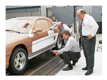
**Figure 5.47 Physical mockups of the mechanical design**(Courtesy of Ford Motor Company.)
